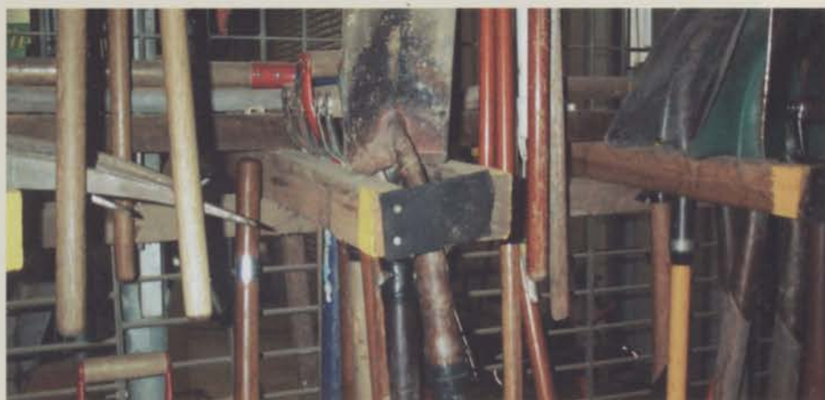
The piece of conveyor belt nailed at one end provides enough tension to hold tools in place when knocked.
