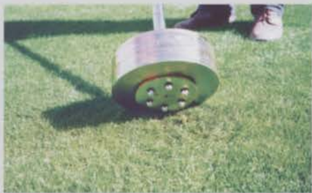
Melbourne researchers are using a studded boot device to measure rotational strength of AFL playing surfaces
