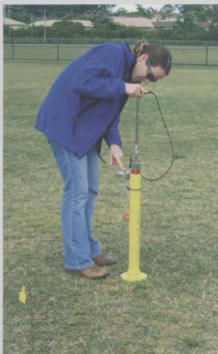
Angelina Gilbert, a team member with the QDPI's AFL playing surface project, measures surface hardness with a Clegg Hammer
