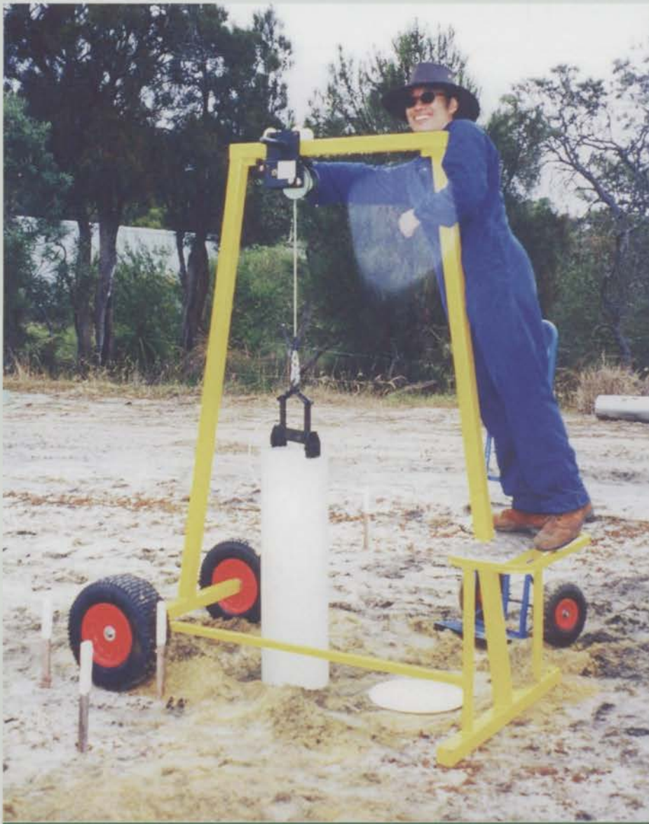
Lysimeters being installed into plots prior to establishing turfgrass
