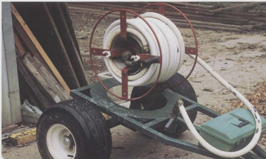
The trailer mounted hose reel which spins 360 degrees
