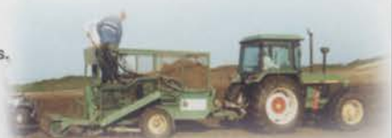
Line planter in operation at Ocean Course, The National, Cape Shank.
