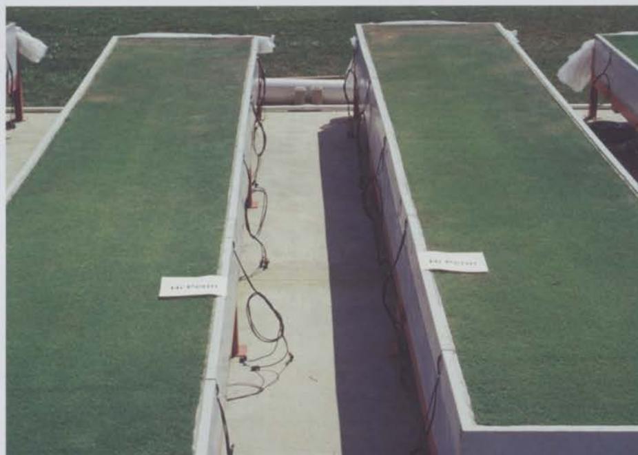
The higher permeability, one- and two-tier putting greens oriented to 4 per cent slope after 10 days without rain or irrigation. Turf in the foreground (downslope) does not show drought stress where turf in the background (upslope) does.
