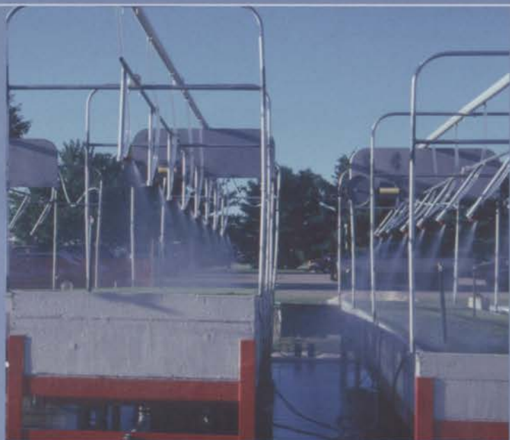
Ohio State University researchers constructed putting greens in elevated tables to investigate the effect of slope, rootzone profile and rootzone mix in the drainage characteristics of water applied at high rates.
