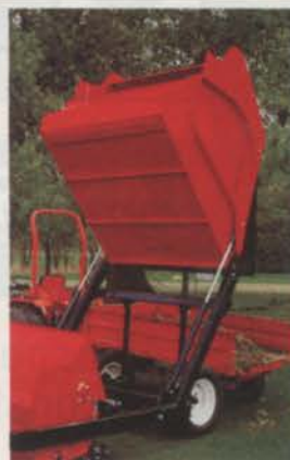
HIGHLIFT – to 2,2 m. enables the operator to discharge into trailers.
