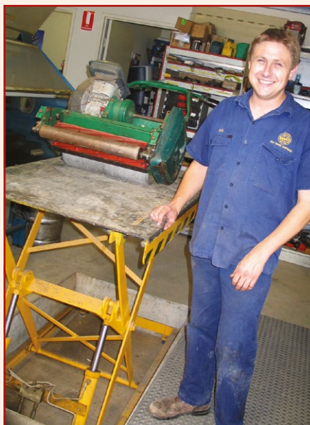
Improvements that Paul Coglan has made to the Avondale workshop, such as this hydraulic lift table, makes everyday work easier
