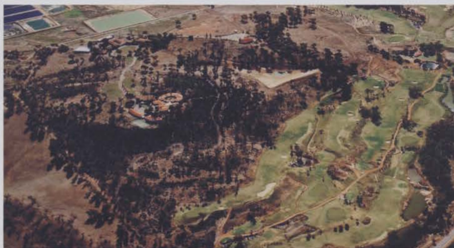
The El Caballo Golf Resort set up which included 10 hectares of effluent treatment ponds, storage dams and three kilometres of open rock drains
