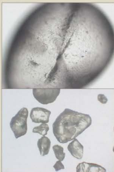
Microscopic images of sand grains indicating variability in sphericity and roundness. (try matching them up with the chart on page 36).
