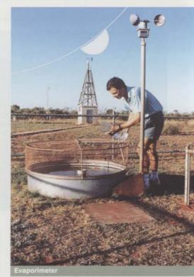
evaporimeter at a point on your course that is typical of most of the course. If water is frequently in short supply, or if you are using effluent water, I strongly recommend that you install an evaporimeter. By using it as I show
