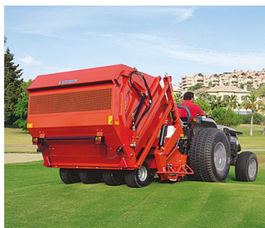
Super 500 Scarifier/Collector to quickly and efficiently remove thatch and dump into a truck.
