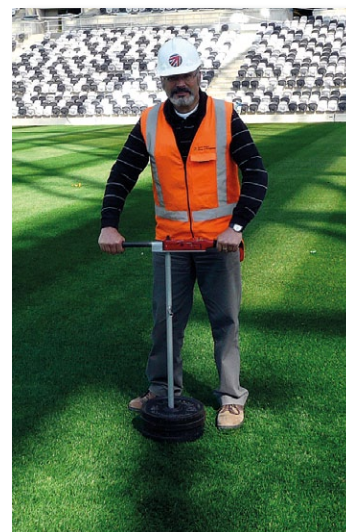
Dr Richard Gibbs undertakes surface traction testing
