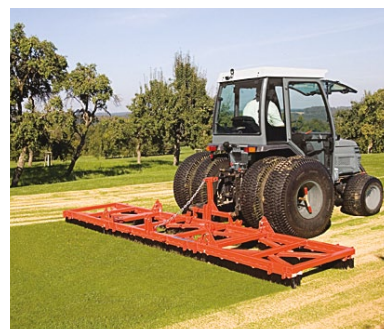
Terra Brush or Drag brush available in 1.8 meter or 4.2 meter versions. Linkage or Trailed.
