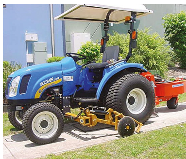
Ezi-Edge Path or Kerb edger. Reduces time and man hours when equipped with a Wiedemann Blower to remove the cut material.
