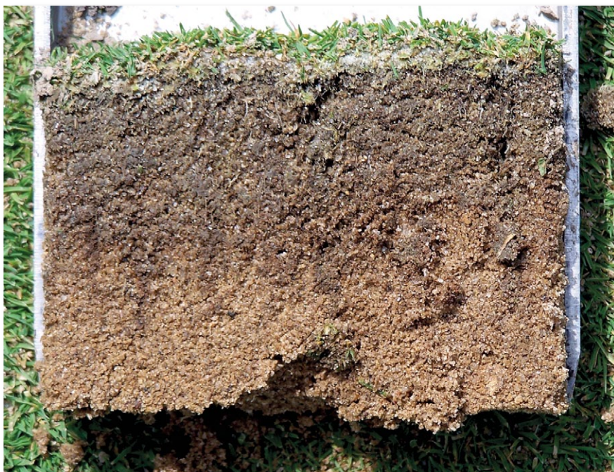
◀ Prior to start of the study, analysis of four randomly selected cores revealed a thatch/mat layer 0-2" deep with 5.8 per cent organic matter
