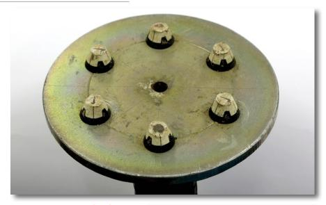
There are several devices in use around the world to measure rotational traction, but the most commonly used is the studded boot apparatus
