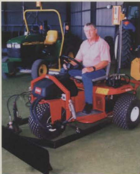
Malcolm Williams aboard his modified Toro Sand Pro bunker rake that has been equipped with laser grade control and dirt shifting functions
