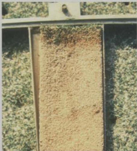
This rootzone profile is of a one-year-old putting green showing the organic matter build-up near the surface.
