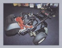
The MT2000 trailer accommodates most Walk Behind Mowers from John Deere, Jacobsen and Toro plus others in either single or multiple chains of mowers.
