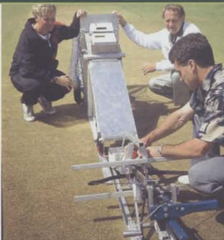
Keith McAuliffe demonstrates apparatus used to measure pitch pace
