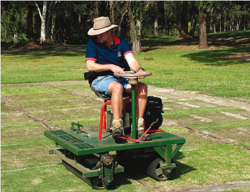
The DEEDI Wear Simulator in operation at Redlands Research Station
