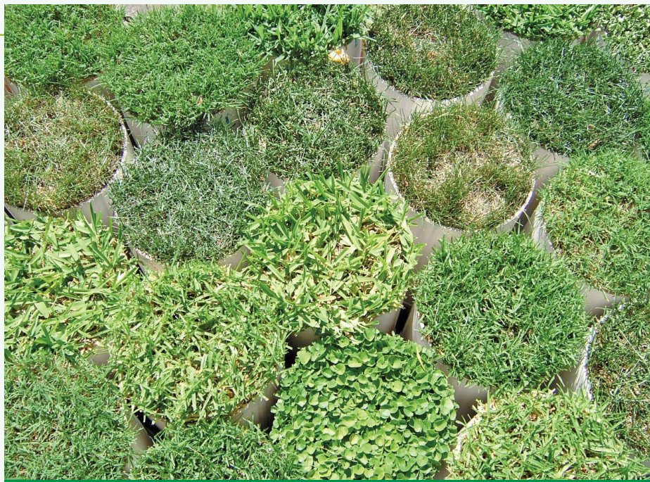
The trial, conducted over the summer of 2005/06, tested water use for a range of turfgrasses commonly used in Victoria. Ten turfgrass species were grown in PVC pots with a diameter of 150mm and a depth of 265mm
