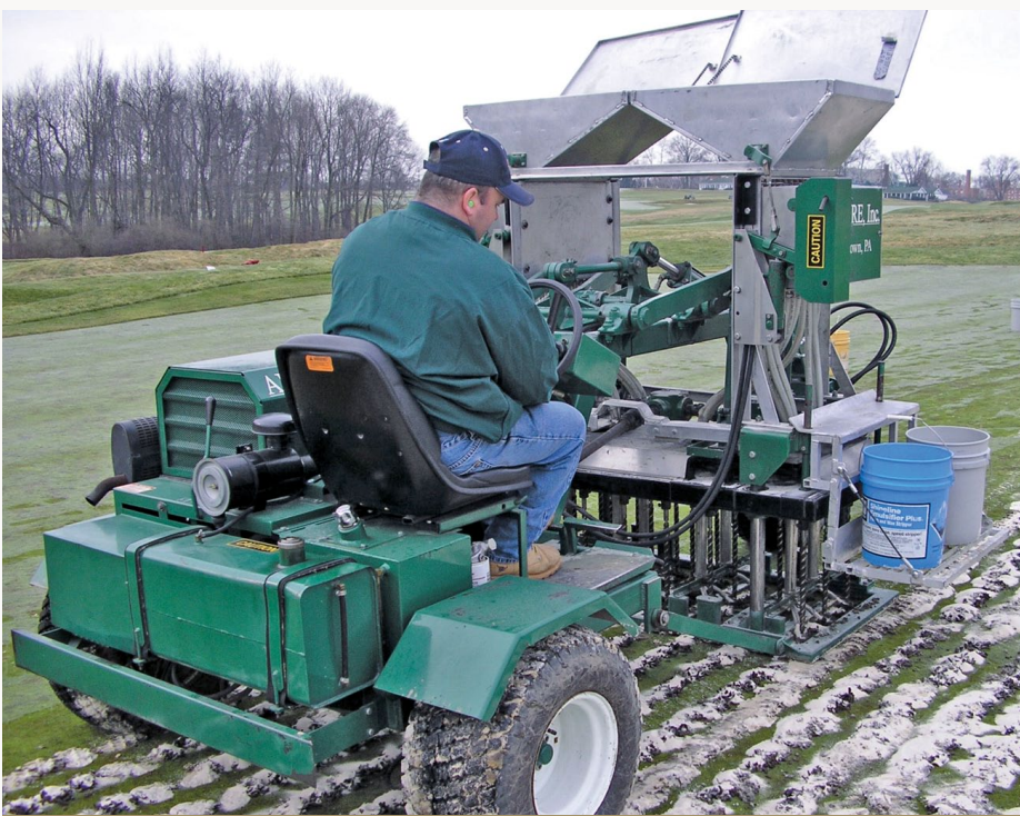
Among the renovation practices used at Oakmont is 'drill-n-fill', where 12-inch (30cm) holes are drilled down to within inches of the sub-surface drainage lines to promote deeper root growth and superior drainage
