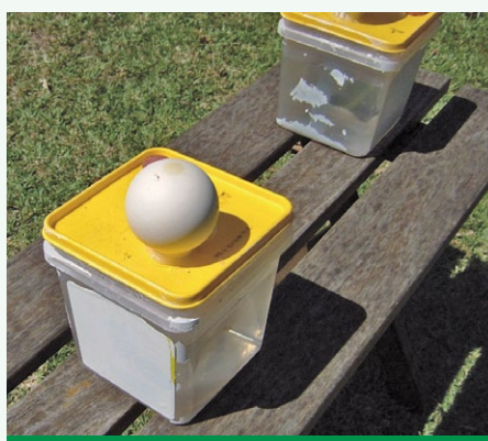
A Livingston atmometer mounted on a water reservoir
