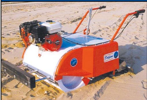
The Delfino Walk Behind Sand Cleaning Machine is a versatile and compact sand sieving machine ideal for even the dirtiest of bunkers. You won't need to replace the sand in your bunkers to achieve a perfect result every time.
