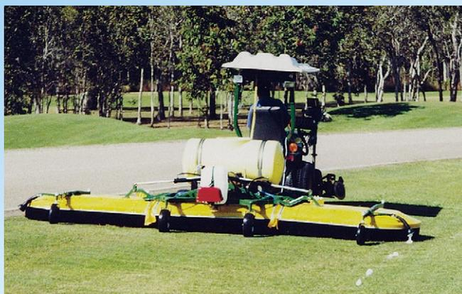
**The new Spraydome 5000 with its ground-hugging, all-round protective skirt means that wind drift is virtually eliminated. This allows you to continue spraying, even on windy days, with greater safety and comfort for both your members and ground staff.**
