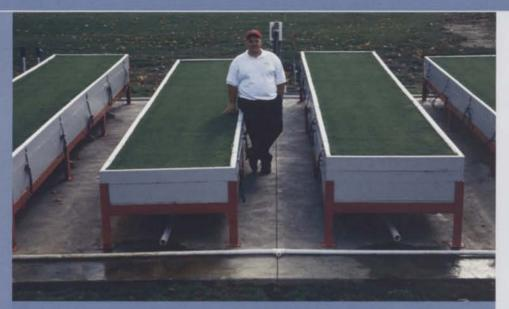
Drainage rates between the two root zone profiles differed significantly. The 2-tier profile greens (right) had a greater drainage rate than the 1-tier greens (left).
