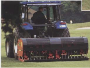
The 3 heavy duty 75-series models Verti-Drain break the compaction up to a depth of 40 cms. These models are robustly built, and do an excellent job when the soil is extremely hard. and contains stones. Corina tines can also be applied.
