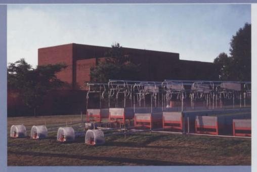
The research greens are constructed within 1.2 by 7.3 meter wooden boxes. The support legs are blocked for slope adjustment, rain simulators are located overhead, and tipping bucket rain gauges are attached to the drainage outflow lines to allow for the measurement of water output.
