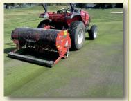
The five greens which were covered in liquefaction were vertidrained to help alleviate silt build up in the profile
