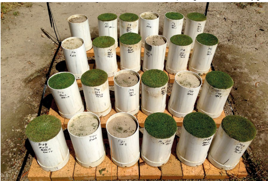
As a follow up to John Neylan's research project on the influence of sand type on surface hardness, a trial was commenced in April 2014 to examine the effects of a turf cover on the hardness characteristics of two different sand types
