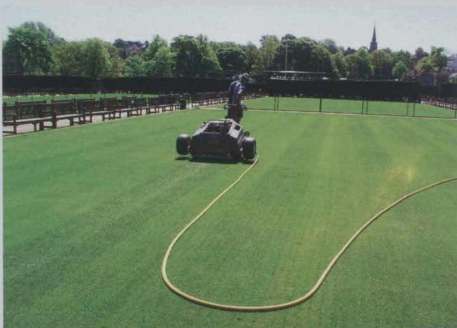
The HydroJect is an effective way to aerate the soil without risking damage to the playing surface or affecting the characteristics of the court
