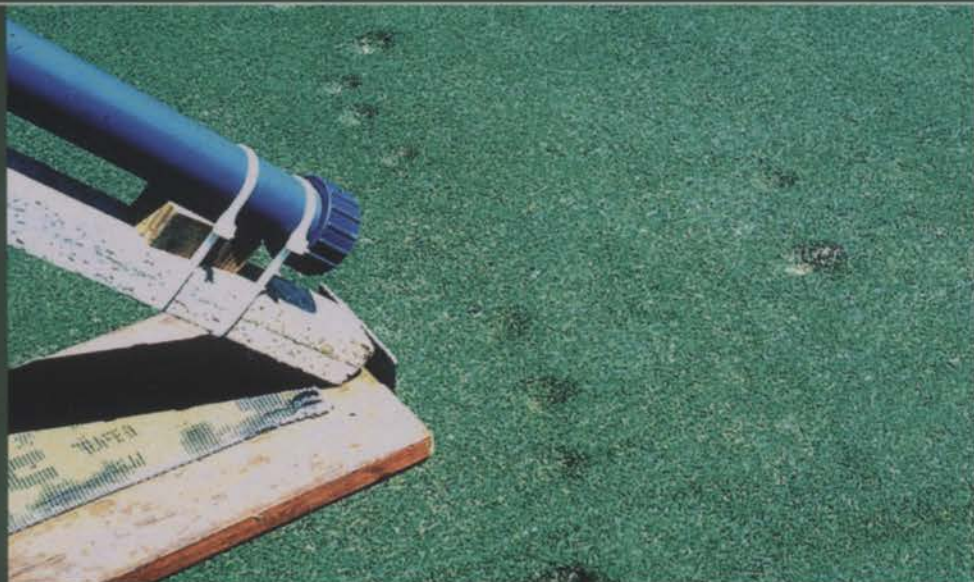
Ball marks were simulated by pneumatically ejecting golf balls from a PVC cylinder at a static pressure of 6, 8 and 10psi. Two to three marks were made in each plot
