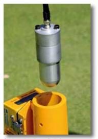
Surface hardness is being measured using a 0.5kg Clegg hammer using both the traditional flat head as well as dome head which mimics a golf ball
