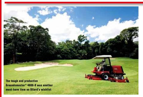
capabilities. It allows operators to trim how they want with one, two, or all three decks engaged, depending on the situation. It also has the SmartCool<sup>TM</sup> system with autoreversing fan which blows chaff off the intake screen to help reduce overheating.
