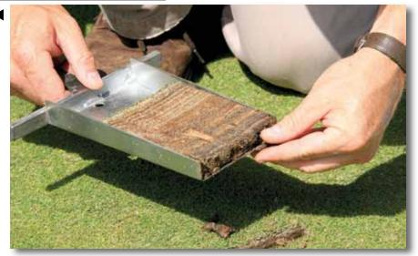
A slice of the upper 150mm of each green is removed with a profile corer to measure thatch/ rootmat depth as well as root depth
