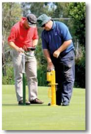
The Trufirm device (pictured left), which measures penetration into the green surface, has been leant to the AGCSA for the duration of the benchmarking study
