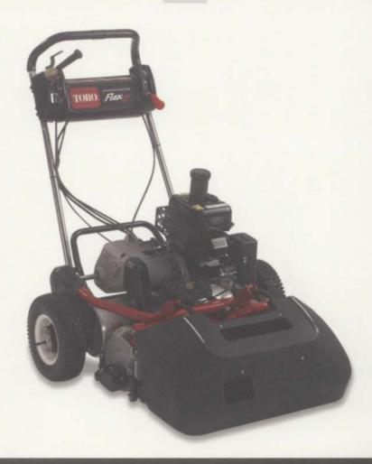
Engine Kawasaki, 4-cycle, 3.7 hp (2.7 kW), air-cooled OHV engine, 3600 rpm. Displacement: 7.57 cu in. (124 cc). Cast iron cylinder sleeve. Electronic ignition. Maximum noise suppression muffler, 83 dB(A) at operator's ear.
