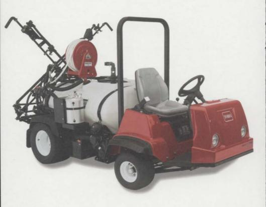
Vehicle 4-wheel, rear wheel drive, front steer, single operator turf sprayer.
