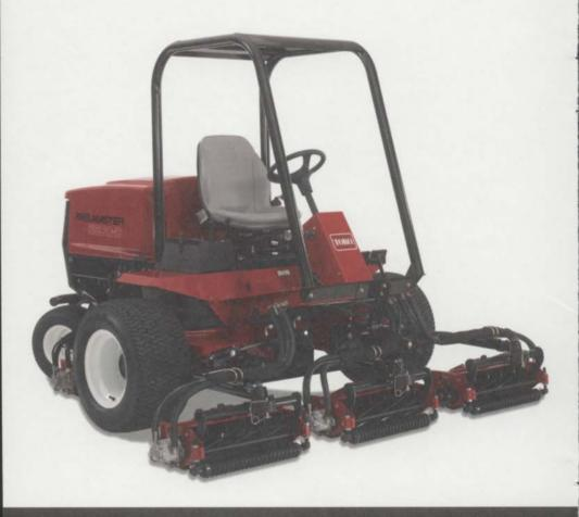
Engine Kubota model V1505T, liquid-cooled, turbo-diesel, 4-cylinder, 46 hp gross @ 3000 RPM, 42 hp net. 1.5 liter displacement. Heavy-duty, two-stage air cleaner with inner safety filter and standard restriction indicator.
