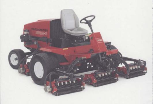
Engine Kubota liquid-cooled turbo diesel, 3-cylinder, 35 hp (26.1 kW) gross @ 3000 RPM, 68.5 cu. in. (1123 cm) displacement. Pressurized lubrication system with 4.0 quart (3.8 liter) capacity. Heavy duty three stage, radial seal air cleaner with dust bowl and restriction indicator. Fuel filter/water separator with visible bowl.
