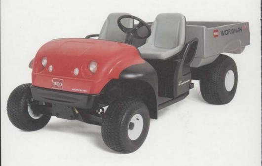
Engine 1100: Kohler 12 hp, single-cylinder: 2100: Vanguard 16 hp, 2-cylinder
