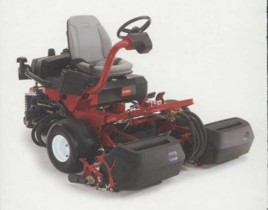
Engine Briggs & Stratton/Daihatsu 850D, 3-cylinder, liquid-cooled, diesel engine, 51.9 cu. in. (850 cc) displacement. Full-pressure lubrication, oil filter. 21.0 hp (15.7 kW) at 3600 rpm. 14.5 hp (12.3 kW) at 2600 rpm. Engine governed to 2750 rpm high idle, 1500 rpm low idle (no load).
