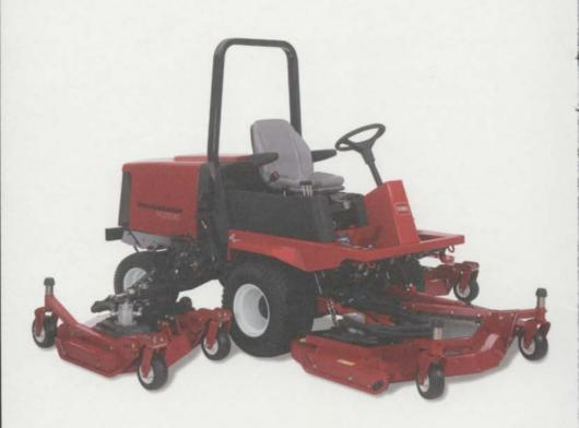
Engine Kubota 2003T, 4-cylinder, turbo diesel, 122 cu. in. (2.0 liter) 60 hp gross.
