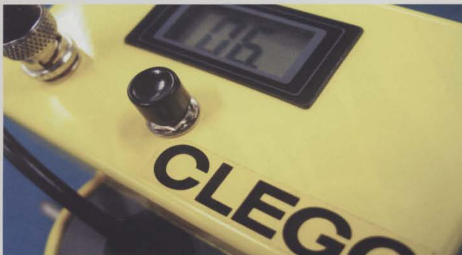
Developed by Dr Baden Clegg, the Clegg impact soil tester measures the 'stiffness' of natural or constructed soils
