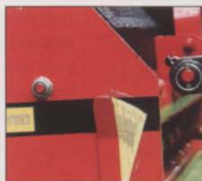
The tine angle lever allows easy fine adjustment to the degree of ground shatter intensity, and quick setting to the vertical position for conventional coring.
