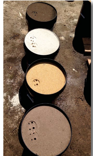
John Neylan's research project is looking at the influence of proportion of silt and clay, moisture retention, moisture release, particle shape and particle size distribution and their effects on surface hardness
