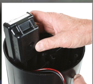
GDC 2-wire module accessible from the top
