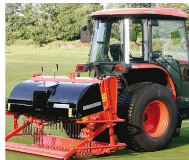
Greens Terra Spike – Deep Tine aerators suitable for use on Greens, Tee's and sand based Sports facilities. No tools required for depth or heave adjustment.
