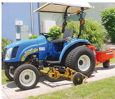
Ezi-Edge Path or Kerb edger. Reduces time and man hours when equipped with a Wiedenmann Blower to remove the cut material.
