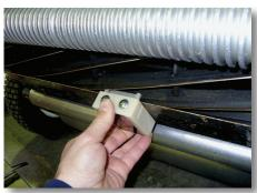
As well as large fully automatic type bedknife grinders there are also smaller less expensive options such as this handheld Bedknife Buddy which has a replaceable file
