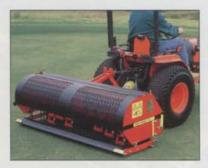
he Verti-Drain Mustang is as fast as a horse, while at the same time it goes deeper than conventional coring machines: 150 mm's.
