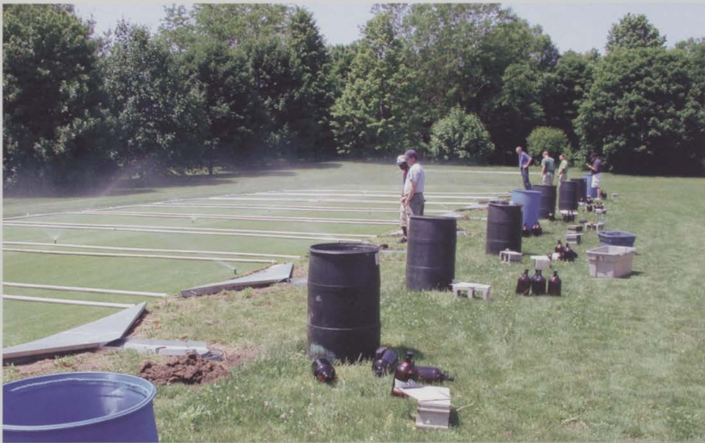
Researchers at the University of Illinois constructed plots to investigate several best management practices to limit pesticide runoff
