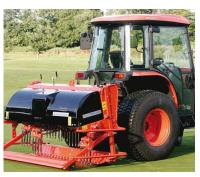
Greens Terra Spike – Deep Tine aerators suitable for use on Greens, Tee's and sand based Sports facilities. No tools required for depth or heave adjustment.
