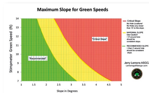
Figure 1. The combination of maintaining fast to very fast green speeds on putting greens with pronounced surface contours results in reduced area for hole locations and increased problems caused by concentrated traffic and wear damage
