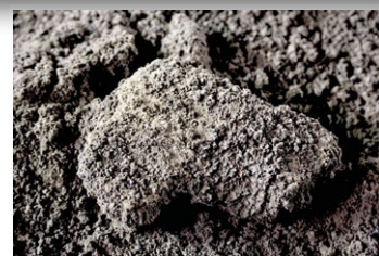
Etihad Stadium's speedway track is constructed using a 25 per cent 7mm crushed rock and 75 per cent silt/clay mix
