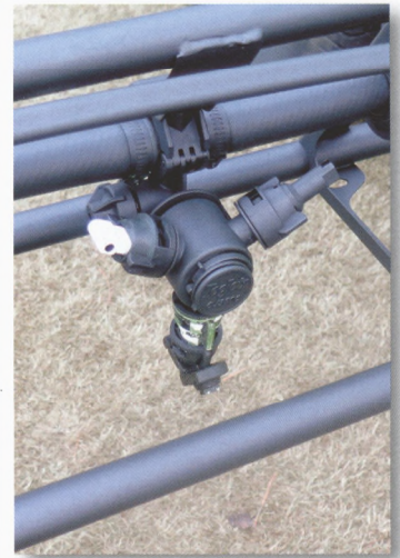
This rotating nozzle body allows course managers to quickly choose between three nozzles, making it easier to use the best nozzle for a specific application
