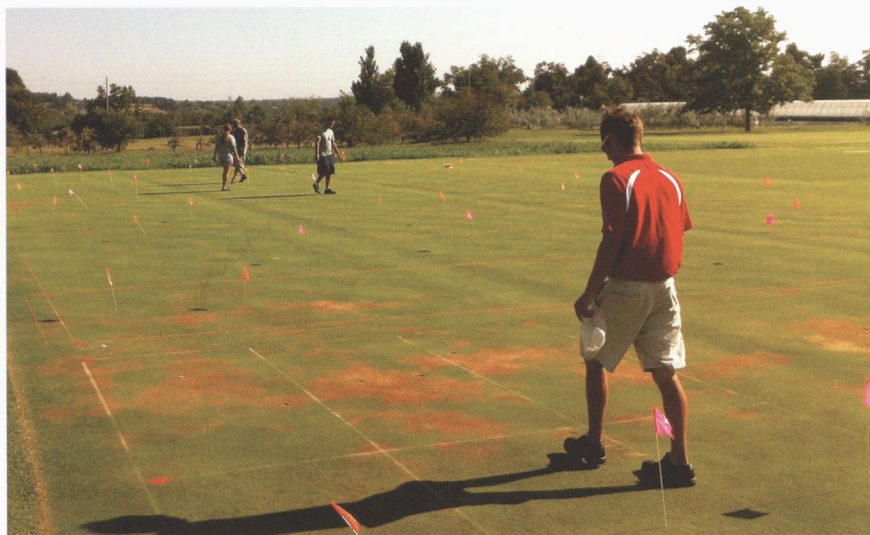
The rolling treatments were split and foot traffic was applied by five individuals wearing golf shoes with non-metal spikes walking within each plot to simulate 200 rounds of golf
