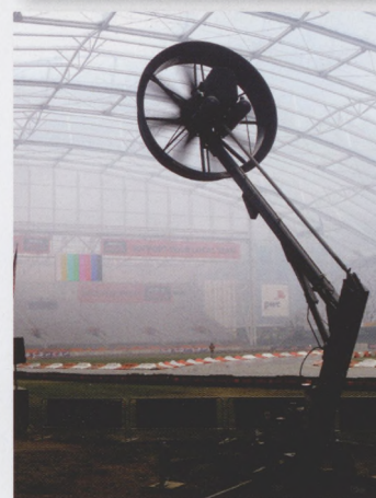
Above: One of the biggest issues was managing the smoke haze created by the cars. Two frost fighting fans from orchards in Central Otago were brought in to help with air movement inside the stadium
