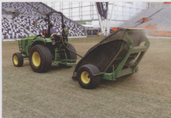
Arena staff used a turf rake and went over the surface multiple times in different directions to loosen up any dead grass and expose the Desso GrassMaster fibres
