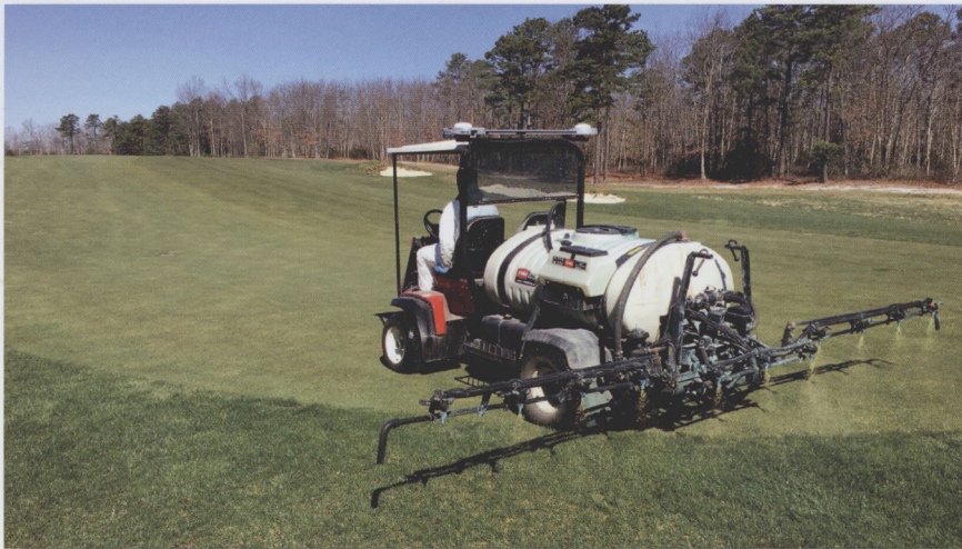
◀ Spraying equipment that utilises GPS technology can improve accuracy and decrease product use
