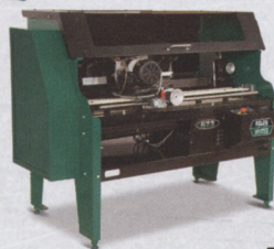
ACCU-Pro 672/673 The World's Most Popular Bedknife Grinder, Auto-alignment & auto angle settings.
