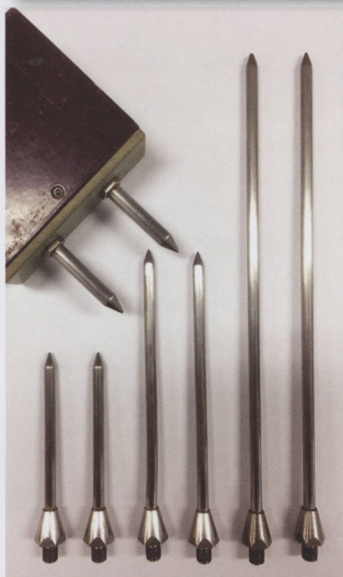
The 7.6cm probe on a TDR probe is a good length for putting greens, with the 3.8cm probes particularly useful for determining the effects of the thatch layer
