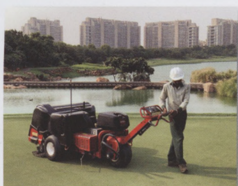
Needle-tying the 5th green in the weeks leading up to the 2018 Hero Women's Indian Open. The greens are Mini Verde bermudagrass
