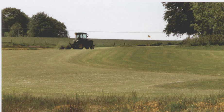
A set of Ransomes 7-knife gang mowers is used to maintain tees and fairways, with an additional 5-knife set for semi-roughs. Both are towed behind a tractor
