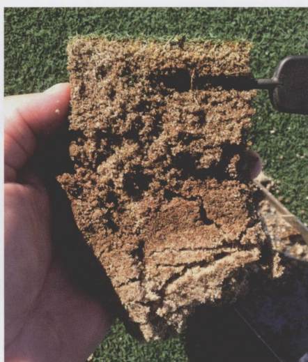
Two growing seasons after initiating a topdressing programme that applied no less than 0.91 cubic meters of sand per 100 square meters annually, organic matter has decreased by 30 per cent
