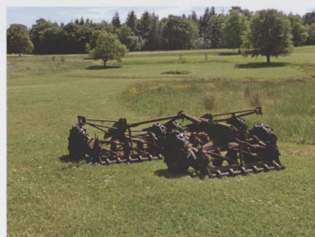
A set of Ransomes 7-knife gang mowers is used to maintain tees and fairways, with an additional 5-knife set for semi-roughs. Both are towed behind a tractor
