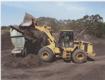
Typically, cricket wicket soil is mechanically excavated from beneath a vegetated surface, screened to size and possibly crushed before storage
