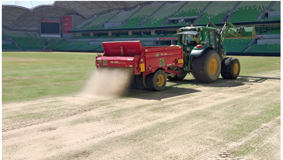
The AAMI Park surface received two topdressing applications of 4mm each prior to and after seeding
