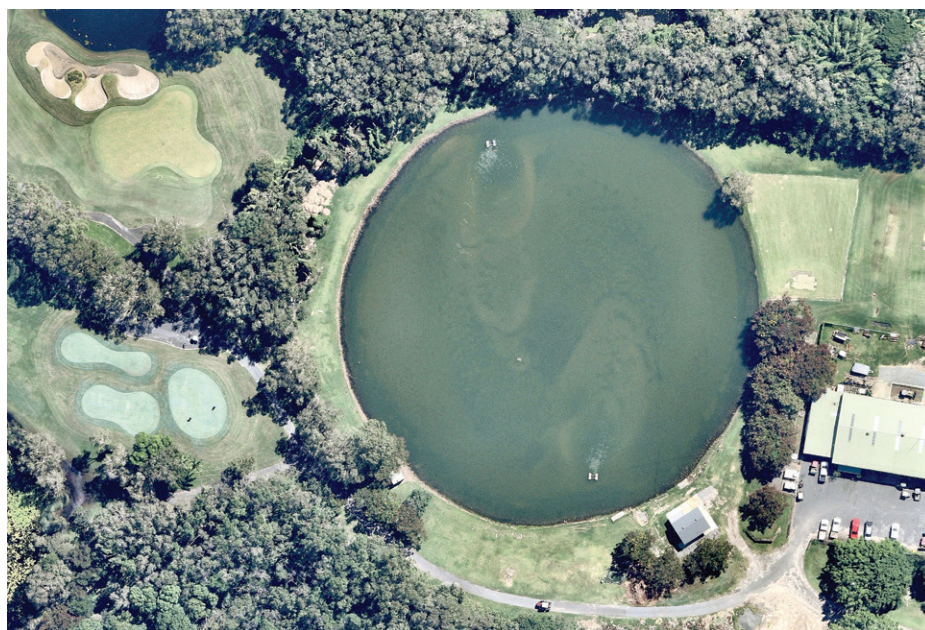
The Twin Waters recycled water storage pond. Note the aerators in the pond for circulation plus Diatomix additive for pond management. Water colour variance is related to oxygen levels, reactive silica, nutrient and algae loads. The new pump station and dosing system shed can be seen bottom right
