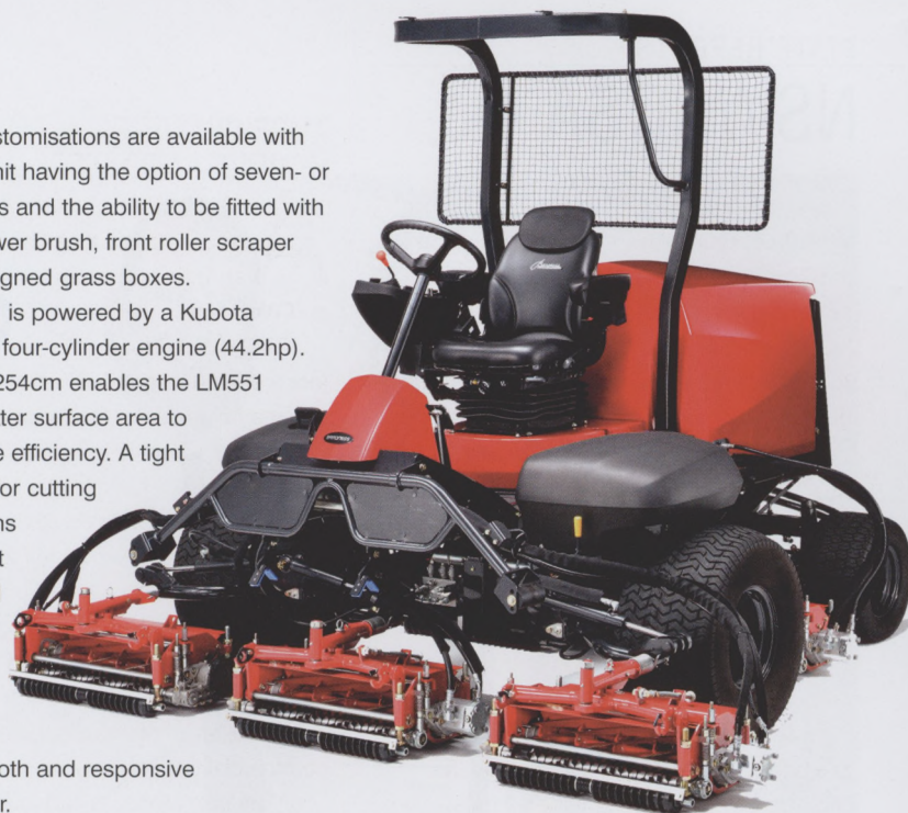
The new Baroness LM551 five-gang mower has been ergonomically designed with custom cutting unit options
