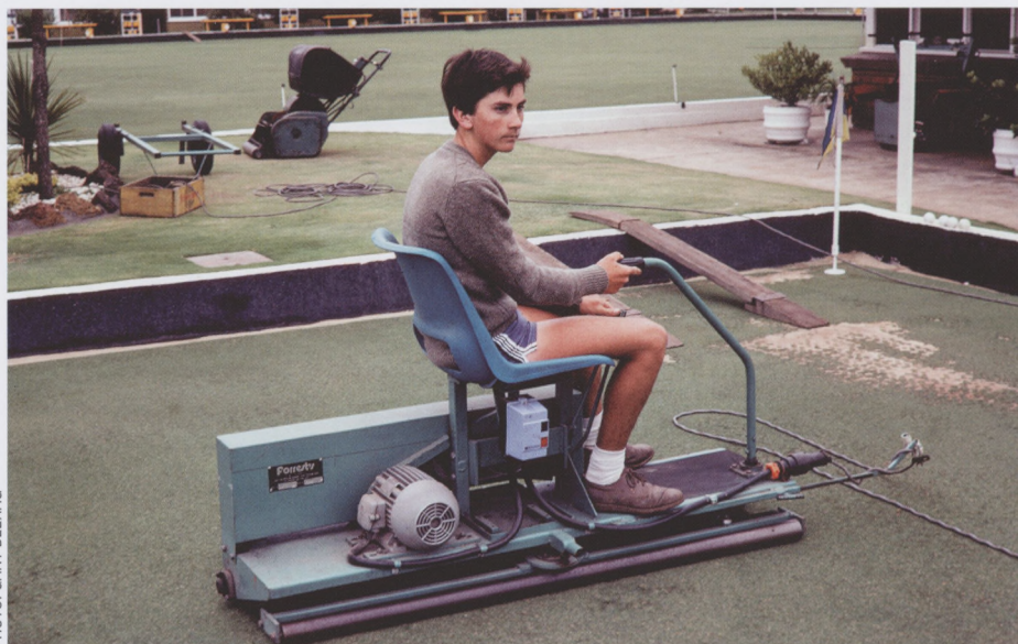
Introduction of the Forrest Greens Roller in 1978 heralded the modern lightweight, multiple-roller for bowling greens
