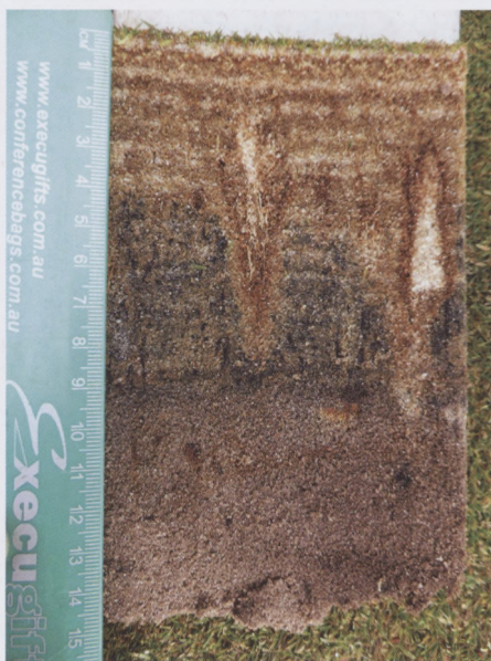
Increased carbon dioxide and hydrogen sulphide levels are toxic to plant roots due to a lack of macropores
