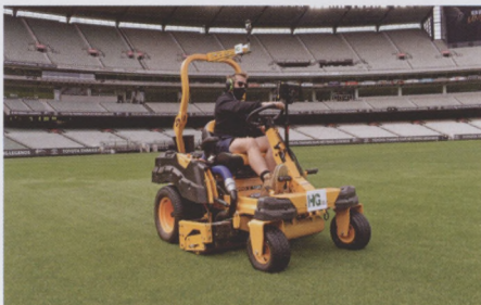
HG Turf's new Turf Print technology uses compressed air to create visual messages and images on turf
