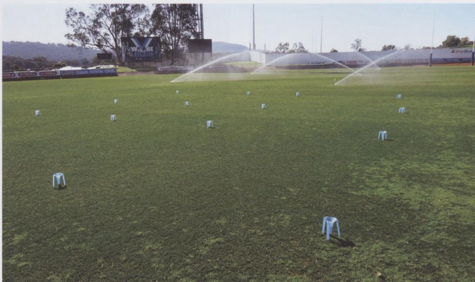
*A catch can audit is an effective way of assessing precipitation rates and distribution uniformity of sprinklers. Such a test should be carried out under 'normal' system operating conditions*
