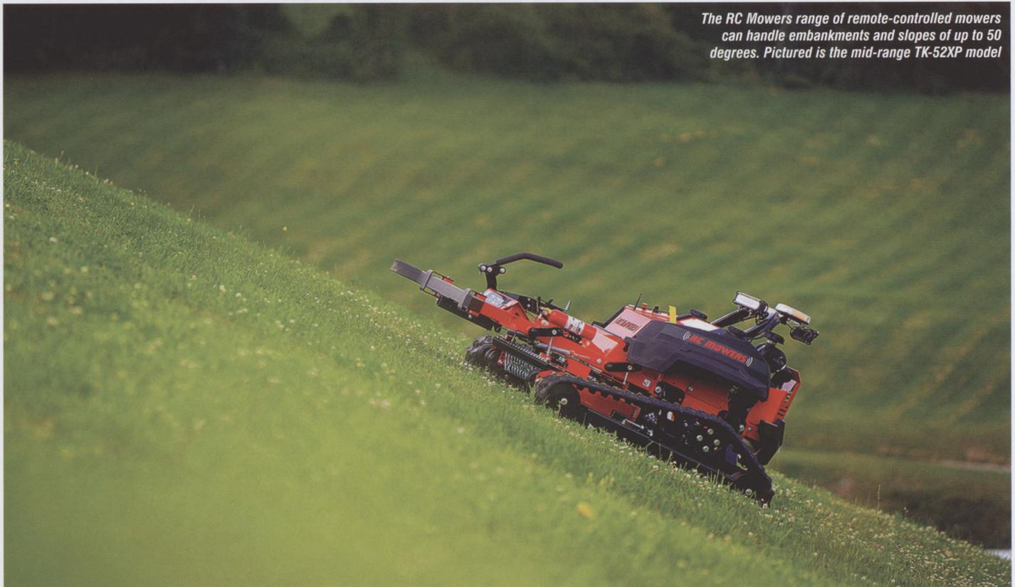
The RC Mowers range of remote-controlled mowers can handle embankments and slopes of up to 50 degrees. Pictured is the mid-range TK-52XP model
