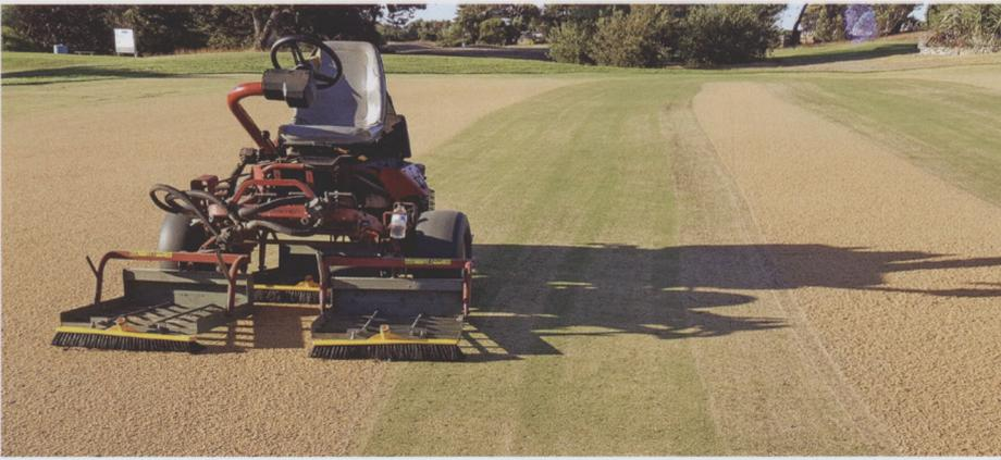
*One interesting piece of kit in the Kingston SE shed is an old Toro greens mower which is used for rubbing in topdressing sand on greens. Three frames were manufactured with broom heads attached*
