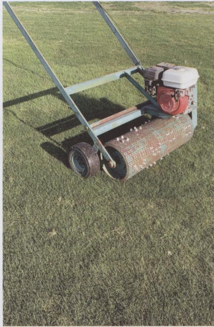
*Wear has been applied to the ANTEP 5 trial plots using AGCSATech's wear machine which consists of 15mm football stops on a rotating drum*
