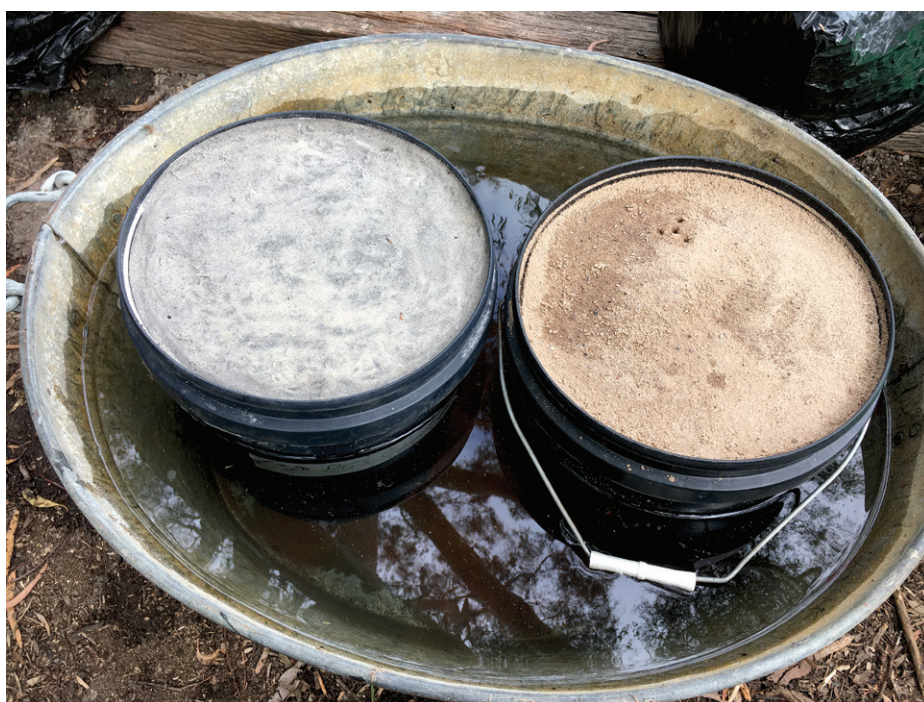
To further explore the relationship between sand type and depth and moisture retention characteristics, a project was established using large containers constructed as a turf profile. Pictured are the samples being saturated by capillary rise
