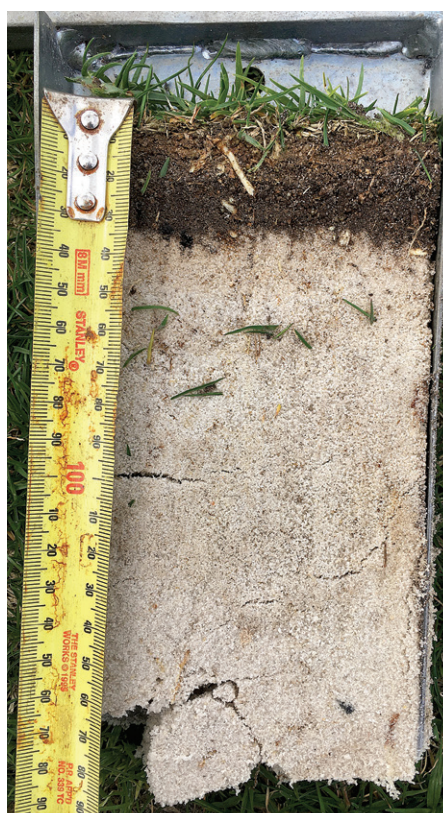
Contamination of a sand drain with poor draining soil and thatch over the surface will reduce the effectiveness of a drain completely
