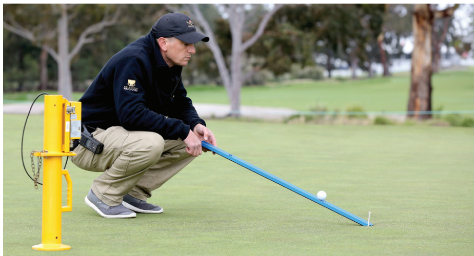
Green speed taken with a stimp meter is a useful measure in understanding the relationship between surface performance and maintenance practices
