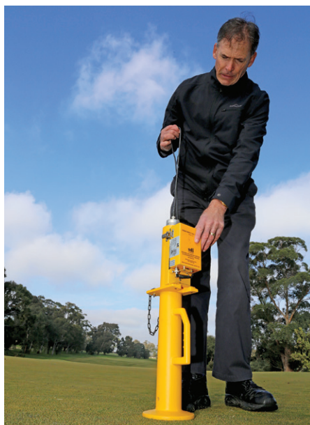
The Clegg Impact Soil Tester is a useful tool to help determine surface variability and whether there are hard or soft areas that could contribute to injury
