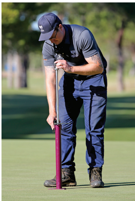
The TruFirm has proven to be a good tool to monitor greens firmness as it changes across the seasons and in relation to soil moisture and surface preparation
