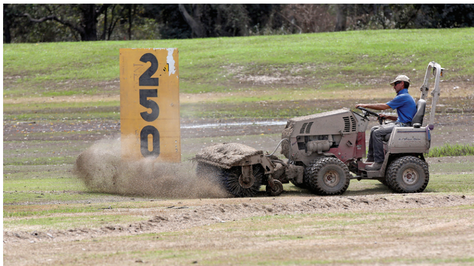
Meadowbrook's Grant Chappel uses a hired Ventrac with power broom to clear off silt deposits from the driving range. All fairways, surrounds, tees and range were cleaned off inside five days
